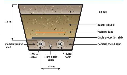
HVDC cables in pairs emit no electric fields due to their metal coverings, and only minimal magentic fields as the current in one cable cancels out the current in the other.
