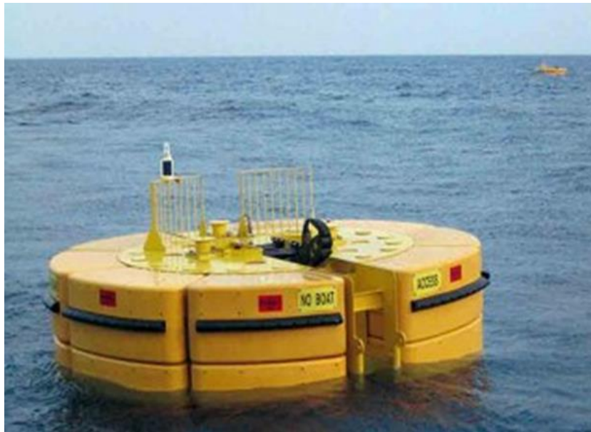
Figure 3.55 Illustrative example of a single buoy mooring
