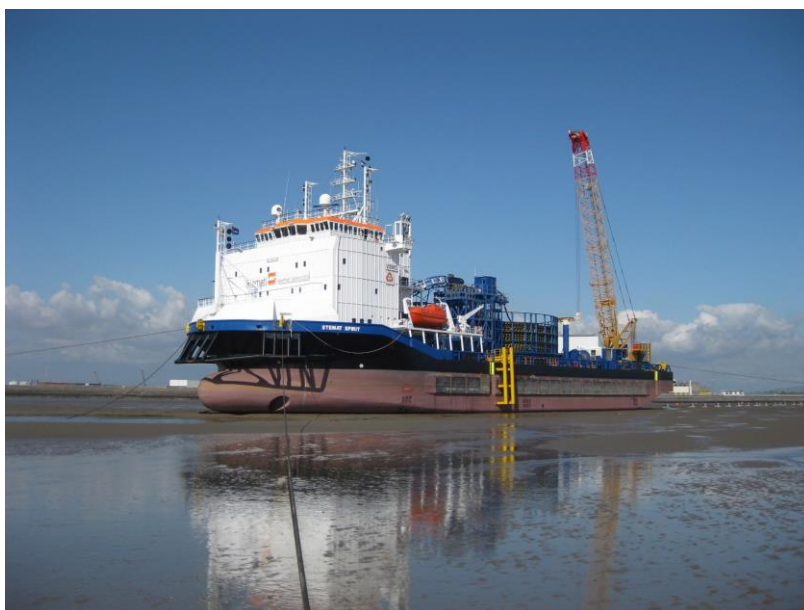
Figure 3.32 Illustrative example of a shallow draft work barge
