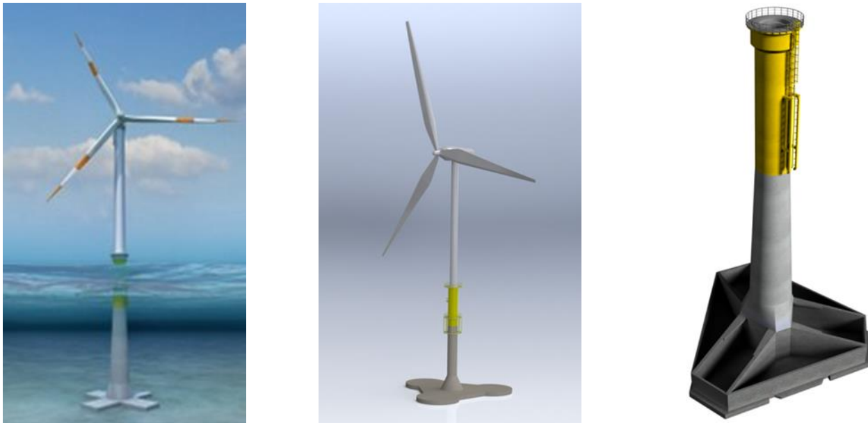
Figure 3.14 Illustrative examples of flat based gravity foundations
