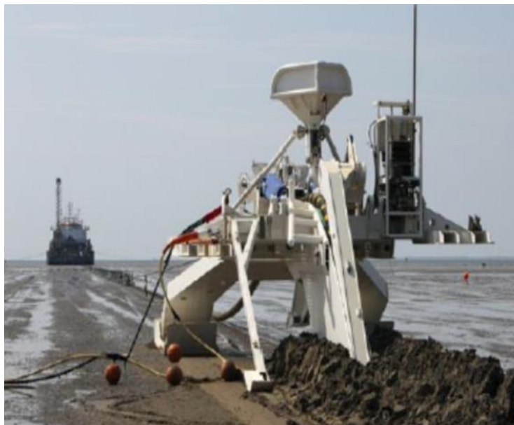
Figure 3.34 Illustrative example of an offshore cable plough
