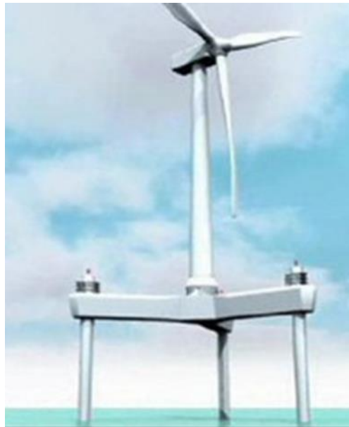
Figure 3.12 Illustrative example of a jack-up foundation
