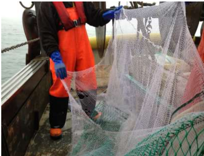
Figure 6. Damaged beam trawl net during the October 2012 inshore survey
