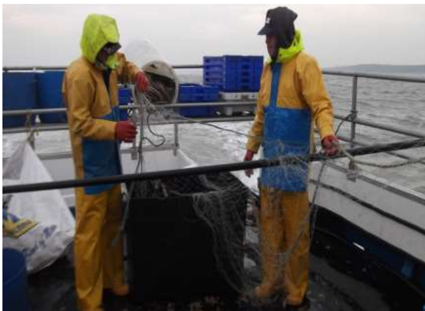
Figure 5. Clearing a fleet of trammel nets into net bin during nearshore survey
