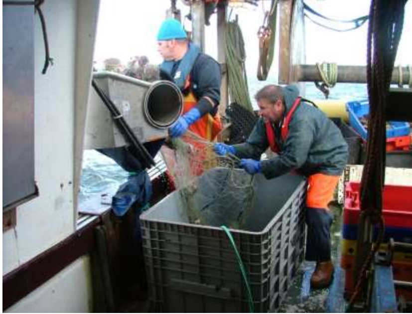
Figure 5. Hauling a fleet of trammel nets into net bin during nearshore survey
