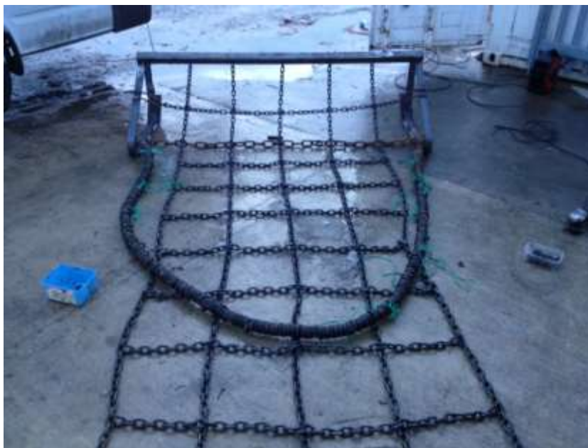
Figure 7. Modified 2-m beam trawl frame without net
