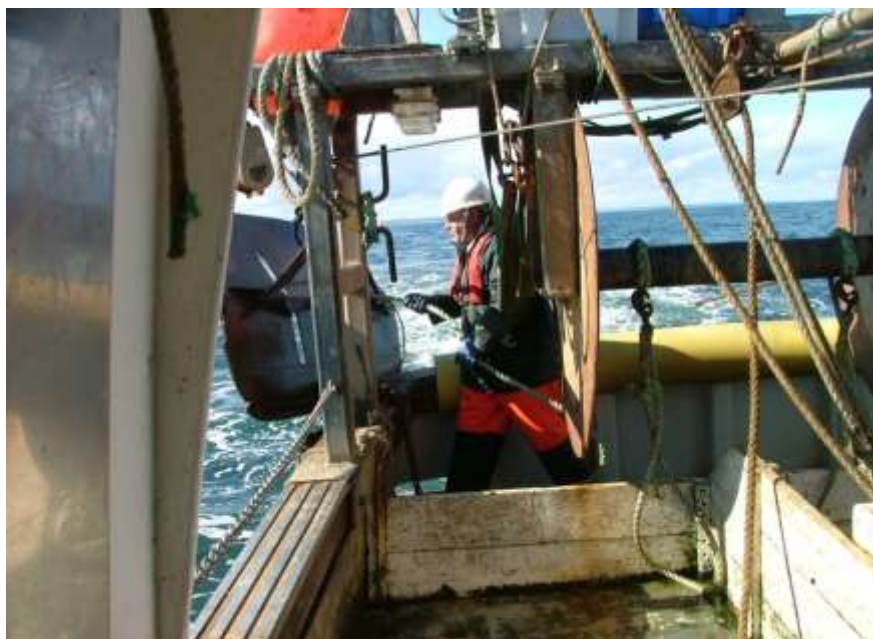
Figure 4. Release of trawl door during prawn trawl survey
