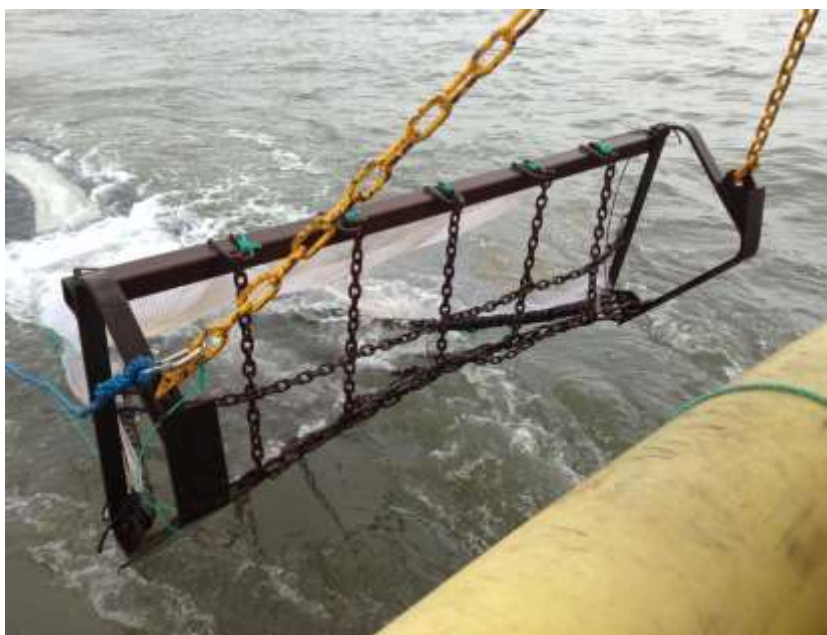
Figure 6. Recovery of modified 2-m beam trawl during the spring 2013 inshore beam trawl survey
