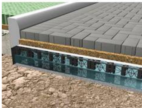
Figure 4 - Section through permeable paving solution indicating storage within a crate system
