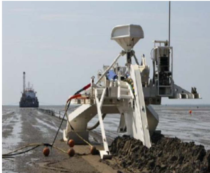
Figure 3.34 Illustrative example of an offshore cable plough
