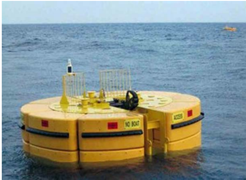
Figure 3.55 Illustrative example of a single buoy mooring
