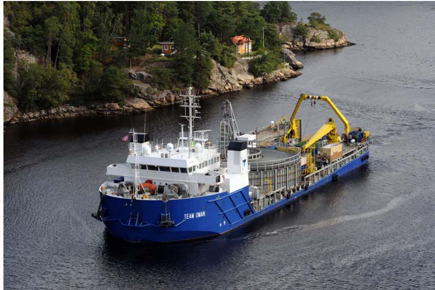
Figure 3.31 Team Oman cable installation vessel
