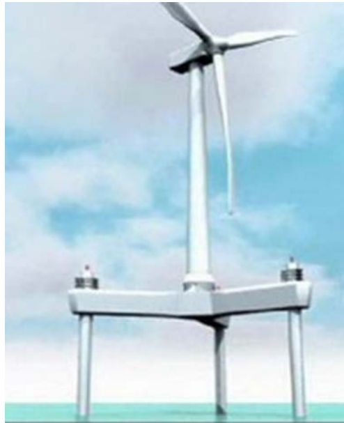
Figure 3.12 Illustrative example of a jack-up foundation
